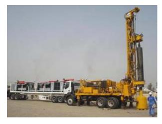
based starting. The unit is also customized with a spark arrestor to prevent fire particles leaving the exhaust pipes. The unique features of the product, in addition to air starting, include emergency stop and intake shut off valve. The unit is powered by KTA 1150 C Cummin s engine for continuous performance in the extreme hot and dusty conditions of the Gulf Region.
